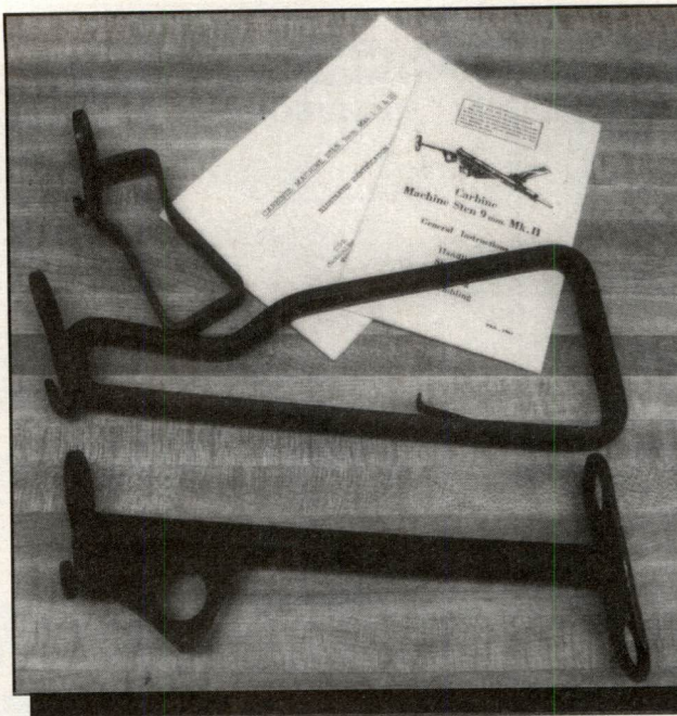
Buttstocks from top: Pistol grip, loop type, "T" type.
