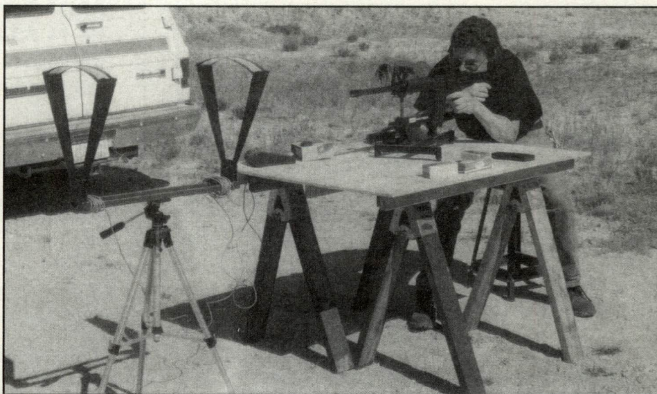
All loads were chronographed using a PACT Mark III timer with chrono and rate of fire option installed.
