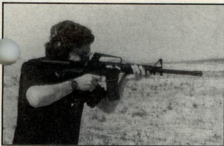
Tom Simpson fires the test gun on semi-auto. Semi-auto fire produces excellent accuracy even out to 100 yards. Recoil is similar to a 12 gauge shotgun.
